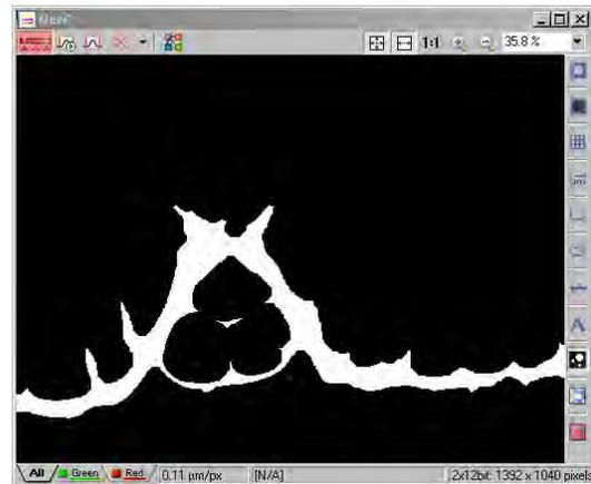
Several Binary processing tools can be used to modify and process the binary layer. These are located in the **Binary** pull-down menu of NIS-Elements. The image above was processed to remove all holes and small objects using the binary functions **Close** and **Clean**.
